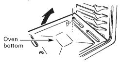
**5.** Locate the pilot in the back of the oven bottom. The pilot is attached to the left side of the oven burner.
